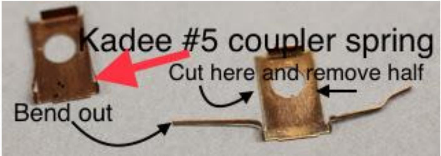
Solder a wire to this and attach to the truck bolster with epoxy. Make sure the axel insulators are on the
