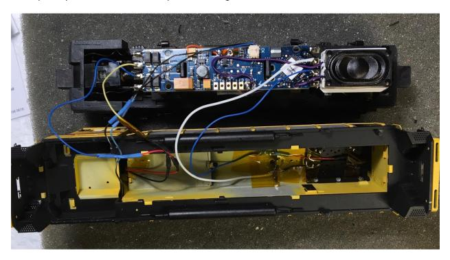
Check polarity of the motor terminals prior to making solder connections!
