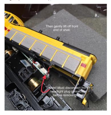
LEDs are connected to the light board and these wires must be disconnected via their plugs before lifting the shell off.
