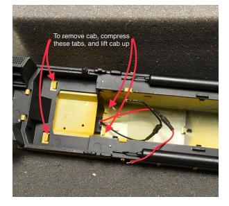
Atlas MP15 DC Switcher Tsunami2 2200 PNP (Note: Double tapping photos in iOS PDF files will enlarge photo) After finally removing the shell this is what you see under the hood!
