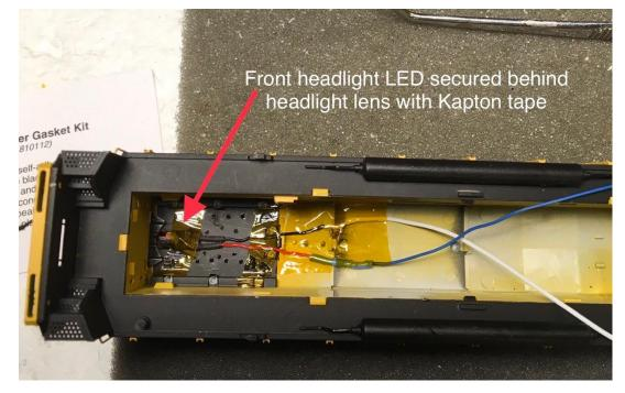
After mounting the decoder we are now ready to make the solder connections to the appropriate solder pads. See the wiring schematic on page 7.
