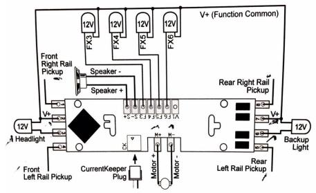
**Note:** This wiring diagram is for use with 12V lights. When using 1.5V incandescent bulbs, connect one lead to the 1.5V Common terminal (V1) and the other to its respective function terminal. Refer to *Technical Notes 17 & 18* for 1.5V bulb and LED wiring diagrams. The TSU-PNP includes a quick-plug for an optional CurrentKeeper (P.N. 810140) to maintain performance during momentary power losses.
