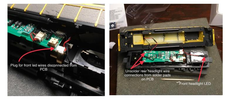
To accommodate the oval speaker I removed the plastic front LED support structure, including the front weight. I secured the front headlight LED to the roof of the shell. Unsolder the rear headlight wire connections and remove the original PCB lightboard.
