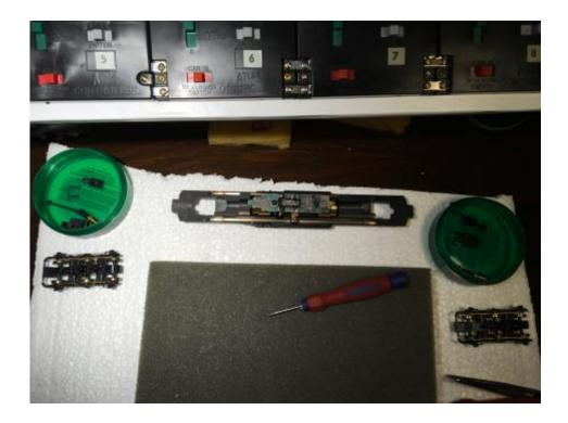
The shell has been removed and the trucks released from the chassis.
