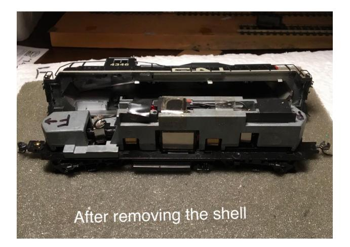
The incandescent bulbs and the diodes are to be removed and replaced with LEDs and resistors. Remove the black tape and plastic covers to access the front and rear headlight wiring. It's always a good idea to label the front and rear of the chassis.
