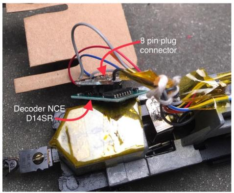
It is good practice to isolate the decoder from any contact with the
