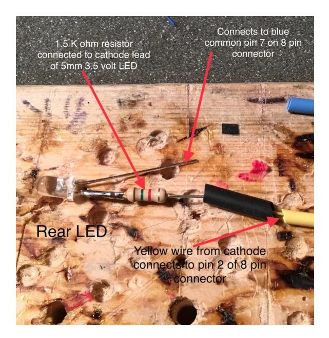
I used white 5 mm 3.5 volt LEDs for the front and rear headlights. The output voltage from the decoder is 12.5 volts so that necessitates using current limiting resistors connected to the negative cathode leads of the LEDs. I tend to use 1.5 K ohm ½ watt resistors, but when space is really limited, I use SMD 1/8 watt 1.8K resistors. (See my previous article "Installation of an NCE D13W Mobile Decoder into a LifeLike GP9 Diesel Locomotive")
