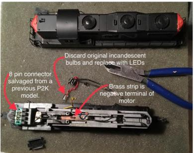
NOTE THE PHOTOS ABOVE DEPICT THE ORIGINAL WIRING as first seen after removing the shell.
