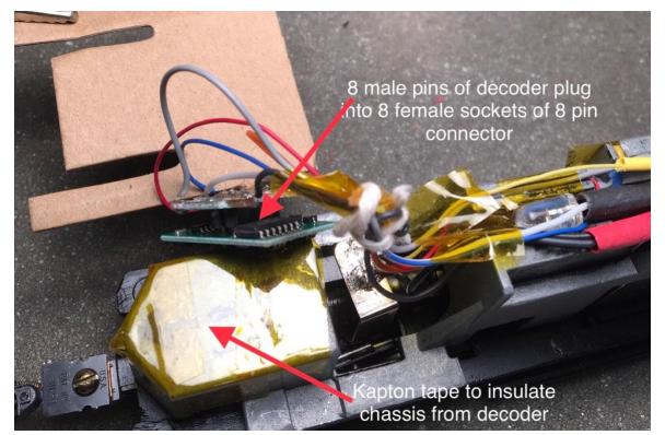
metal chassis by placing Kapton tape on all appropriate metal surfaces.
