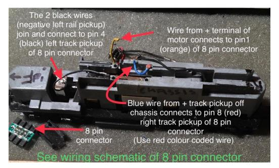
purchased or you can buy the decoder with an included 8 pin harness. The NCE D14SR did not include a harness as it is designed for use with DCC Ready locomotives that have the 8 pin connector already installed.
