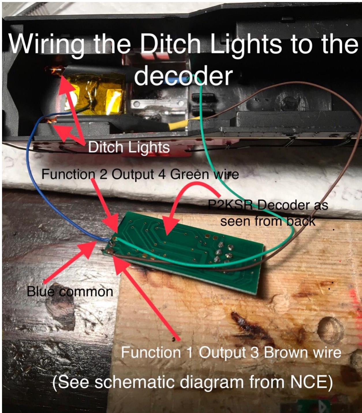
Photo of Decoder board and additional LED connections for Ditch Lights
